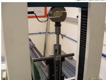
Figure 1. A pull out test in progress.
